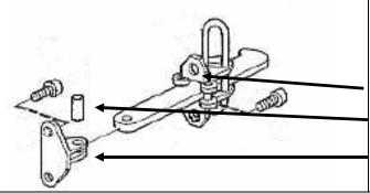
Door Restraint assembly (LH door shown)
