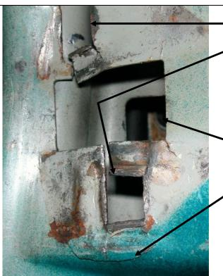
Picture looking into door. The upper retaining square hole has gone with the metal stripped away above. The lower retaining square hole has cracked away with stress cracks appearing at the corner of the stay slot. Out of picture is a fatigue crack over the top of the stay hole.
